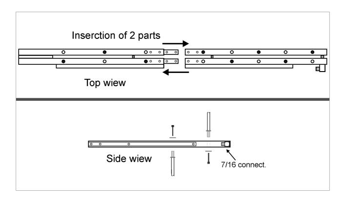
Please, apply spray Oil on all the contact surfaces and the screw holes.
